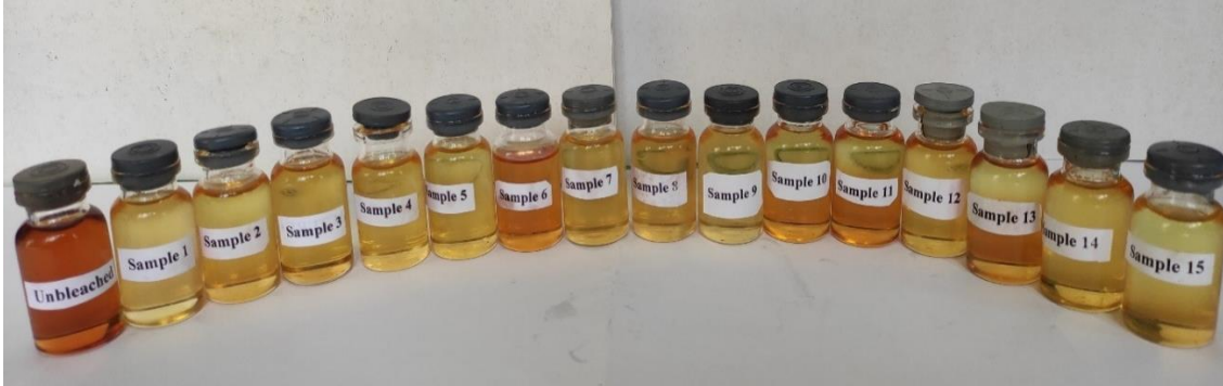
Figure.1. Sesame Oil Before and After Bleaching with Prepared Activated Clay
